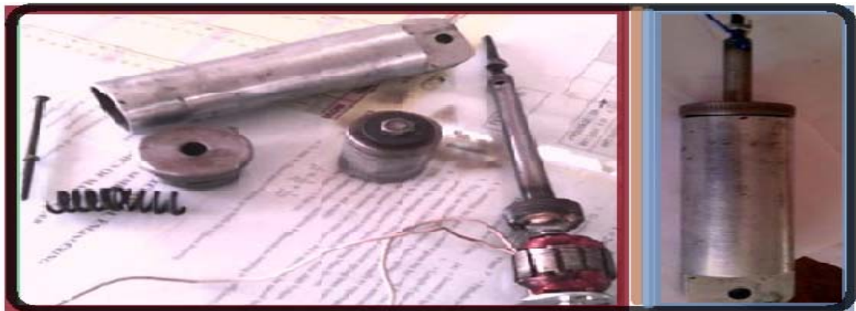
Figure 2: Schematic diagram of fabricated Magnetorheological Damper
