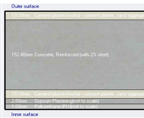
Figure 8: Roof Layer Construction
