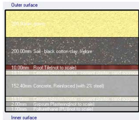
Figure 10: Roof layer after applying ECM Green Roof
