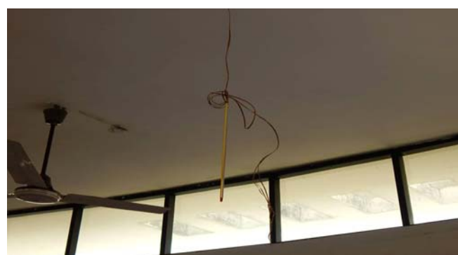
Figure 5: Thermometer put in LT 21 for air temperature measurement
