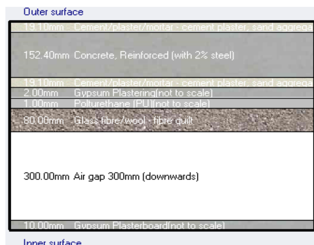
Figure 9: Roof layer after applying ECM Ceiling
