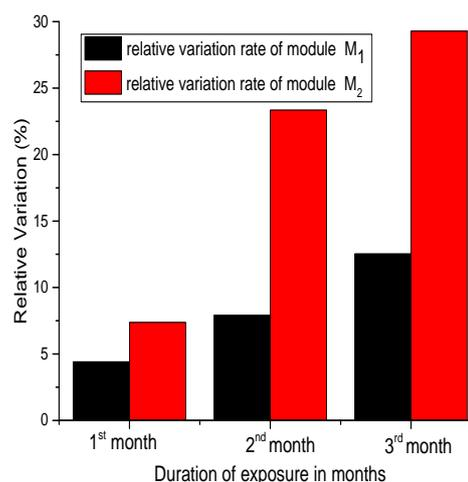
Fig 3. Comparison of the variation rates of the performance of the two modules after three months of exposure.
