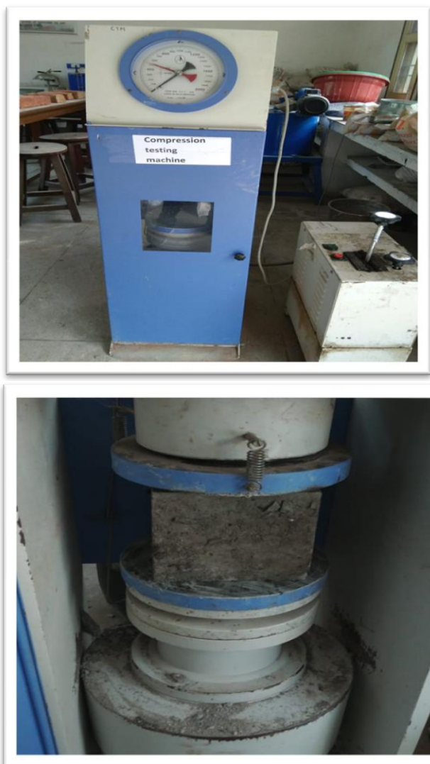
Fig . 9 Specimen loading for compressive strength test
