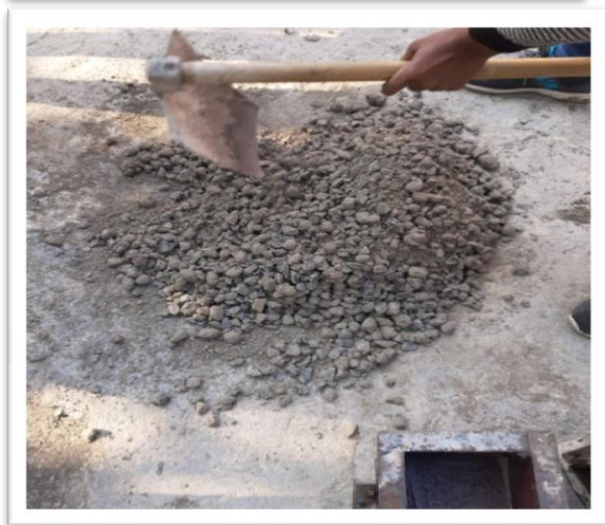
Fig. 6: Casting of cubes
