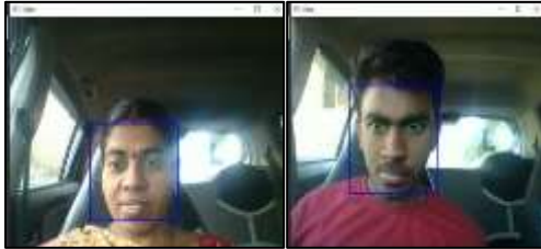
Fig. 5 Driver eye detection using proposed Identifying Eye Aspect Ratio (I-EAR)
