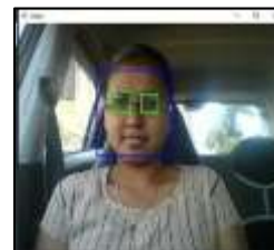
Fig. 4 Real time eye detection with spectacles
