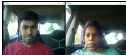
Fig. 2 Real time vehicle driver face detection
