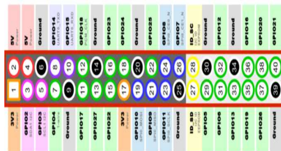
Fig 7. GPIO pin numbering.
