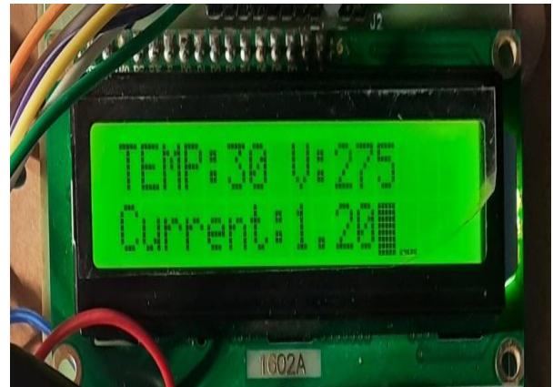
Fig 11. High voltage condition - Output from LCD screen.
