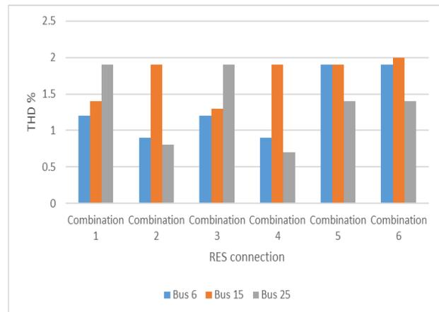
Fig 3. THD (%) at PCC for the six combinations.
