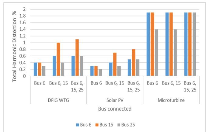
Fig 1. THD (%) at PCC after integrating RES of same type and capacity (increasing penetration level).
