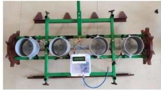
Fig.7[i]. Implementation of seed counter
