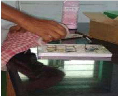
Fig.6 Pouring of PCM to back side of the panel
