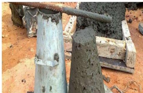
Fig 3. Slump cone test
