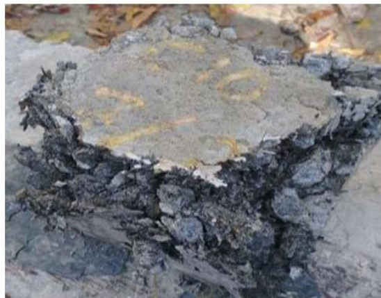
Fig 5. Failure of cube RP 5 It is observed that, compressive strength decreases as the rubber percentage increases.
