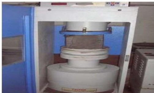
Fig 4. Compression test on concrete cubes.
