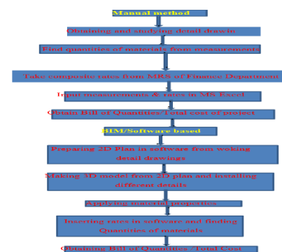
Figure 2: Compare cost estimation by Manual/BIM based software
