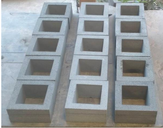
Fig. 1 □ The ventilation blocks with mixed TiO 2 (a) 2% wt , (b) 4 %wt and (c) 6 %wt
