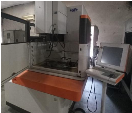
Figure1 EDM used during machining of AMMCs
