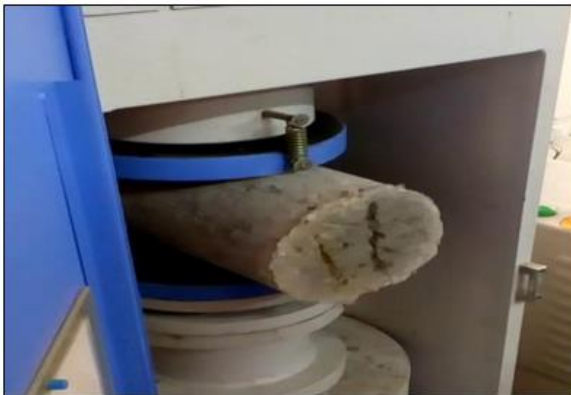
Fig 3 Split Tensile Strength.
