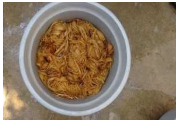
Figure 1 Banana Fiber with NaOH Solution
