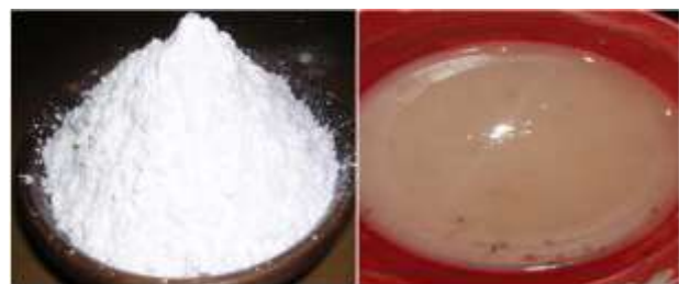
Fig. 3: Cassava Starch Powder and Cassava Starch binder solution
