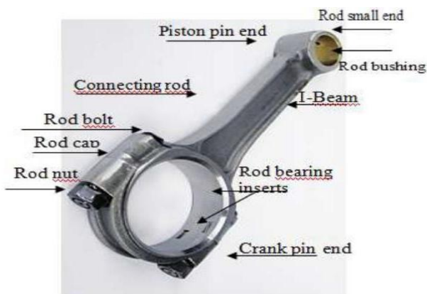
Fig 1. Different parts of connecting rod.
