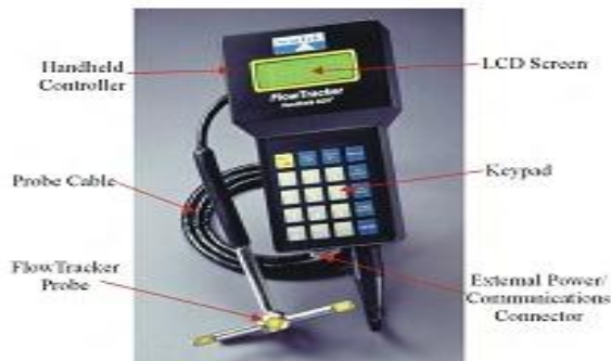
Fig 5. Plate (4) The Flow Tracker with all major components labeled.
