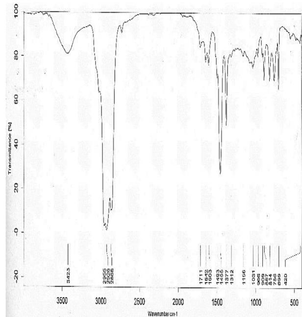
Fig 3. Infrared spectra of the obtained liquid product.
