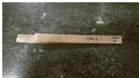
Fig 11. Composite sample after tensile test (sample1).
