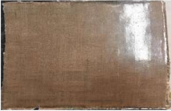
Fig 7. Composite specimen from compression moulding machine.
