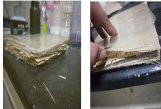
Fig 4. Jute/Bamboo PLA arrangement before composite formation.
