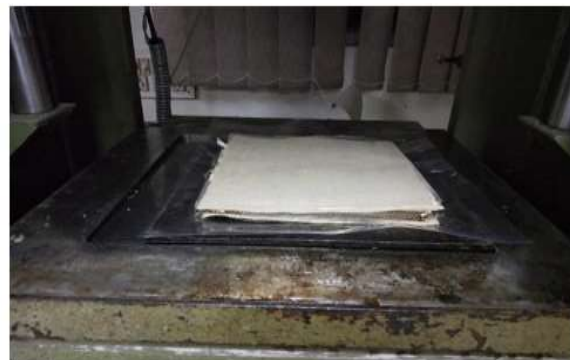
Fig 5. Arrangement of Jute/bamboo/PLA inside compression moulding.
