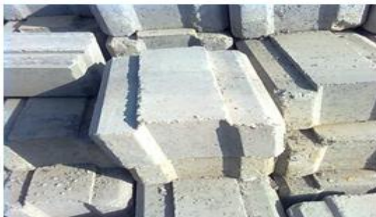
Fig 4. Interlocking Brick (Ridge).
