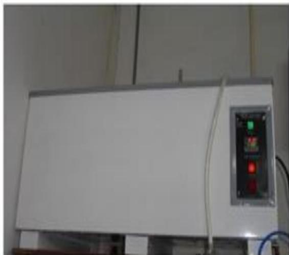
Fig 3. Constant temperature water supply bath.\
