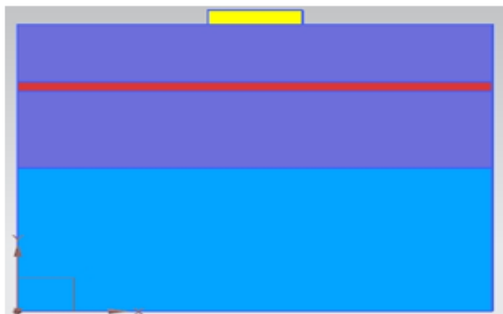
Fig 8. FEM Model of foundation with geogrid at u=300\text{mm} .
