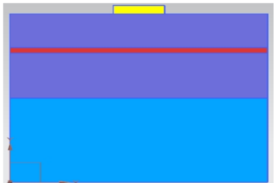
Fig 6. FEM Model of foundation with geogrid at u=0\text{mm} (just below footing).
