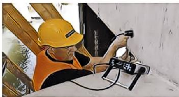
Fig 4. Ultrasonic Pulse Velocity.
