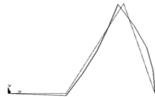
Fig 10. Third mode shape of flexible four-bar mechanism for \theta_2=0^\circ .
