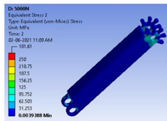
Fig 2. Stress plot (base model).
