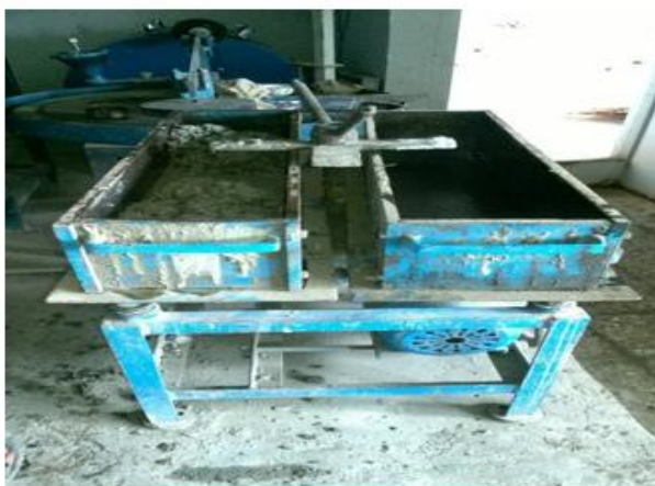
Fig 1. Vibration and costing of beam 150mmx150mmx150mm.
