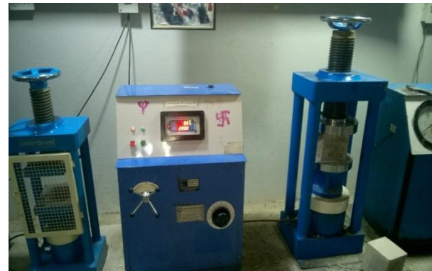
Fig 2. Compression testing machine or cube test.
