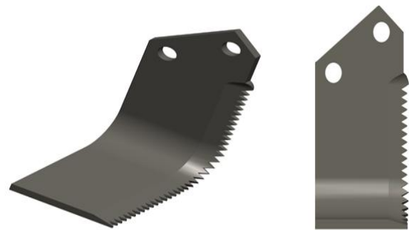
Fig 3. Modified Rotavator Blade with saw teeth.
