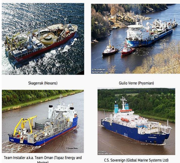
Fig 3. Specialized vessels for cable laying at sea; owner mentioned in the brackets https://electrical-engineering-portal.com/wp-content/uploads/2017/09/trench-sea-power-cable.jpg
