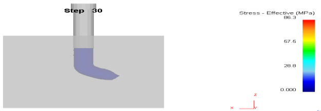
(c)Channel angle ( 120^\circ ) and corner angle ( 20^\circ )
