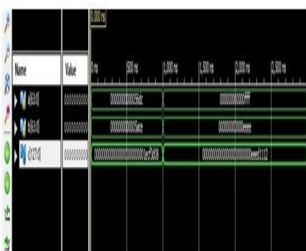
Fig 4. Test bench results in hexadecimal.
