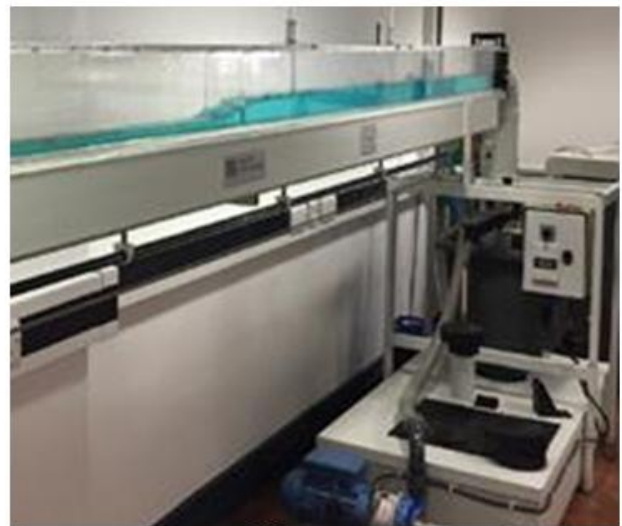
(b) 5m flume with the discharge measurement apparatus.
