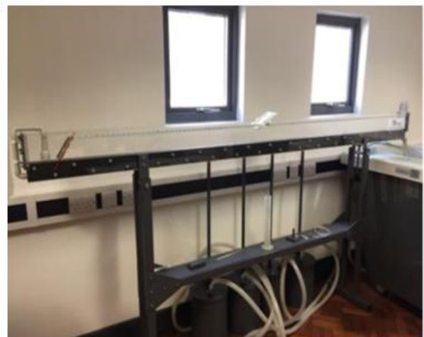
(a) 2.5 m flume used in experimental work.
