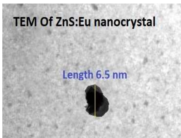
Fig. 4 HRTEM image of 2 mol% Eu-doped ZnS nanocrystals
